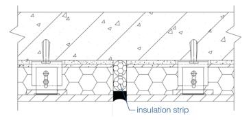
After the application of insulation stripe, the depth of the panel joint left for the application of sealant shall be no less than 5 mm.
