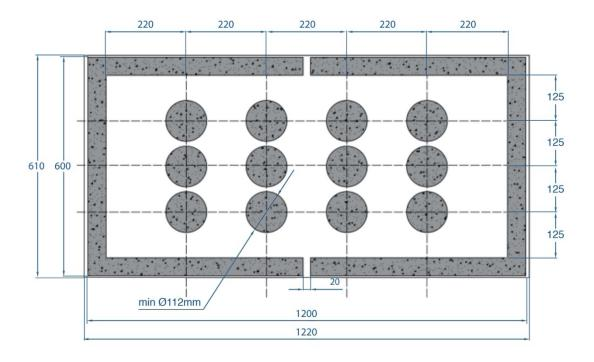
Apply adhesives on the adhering points on the back of the panel, place the panel to the substrate with even force, and adjust it to its precisely designed position with required flatness, before anchors are finally applied.
