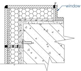
Attention: Number of clips and brackets may increase correspondent to the size of the panel, with minimum 8 clips and brackets within each square meter. Actual number of minimum clips and brackets must be designed to comply with the building wind load requirements.
