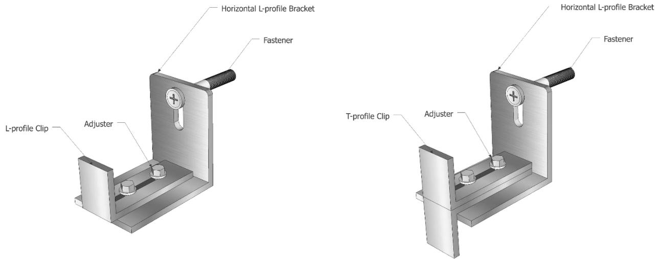
**FIGURE 1—ILLUSTRATION OF A WALPANEL WALLSHELL® LT ANCHORING SYSTEM**
